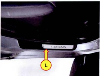
4. Cover front step plate (L) with sponge pad, and then proceed to fasten securely front step plate with **rubber hammer.**
