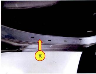
3. Install the new door step plate in reverse order of removal.
