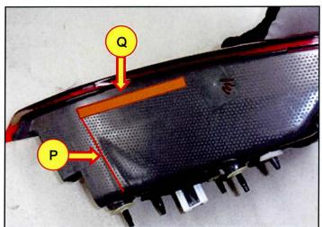
14. Attach the pad to the rear combination lamp for LH & RH and then reinstall all the removed parts in reverse order of removal.
