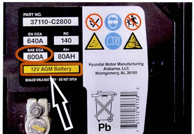
Example of Sonata (LF) AGM Battery Specification Label
