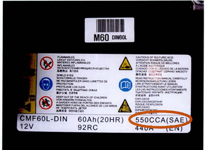
Example of Sonata (LF) AGM Battery Specification Label
