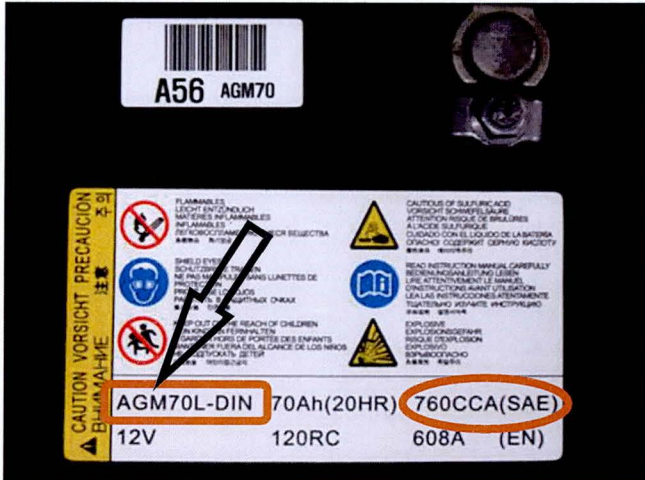
Example of Genesis Sedan (DH) AGM Battery Specification Label
