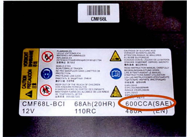
Example of Elantra (UD/MD) Flooded Battery Specification Label
