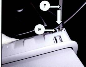
7. Insert the new holder latch (E\*) with needle nose pliers (G) in the orientation shown.
