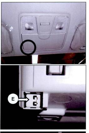
Push the back side of the holder latch (E) with a driver (F) to remove the holder latch from the overhead console.
