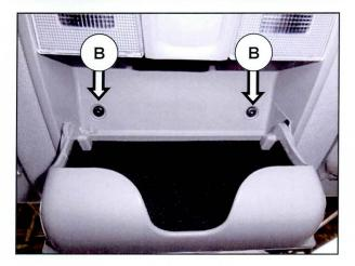
2. Remove the two screws (B).
