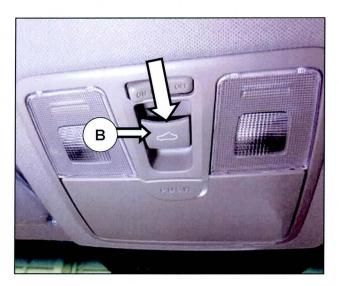
4. Keep holding the switch until the sunroof glass automatically tilts up and then moves up/down slightly.
