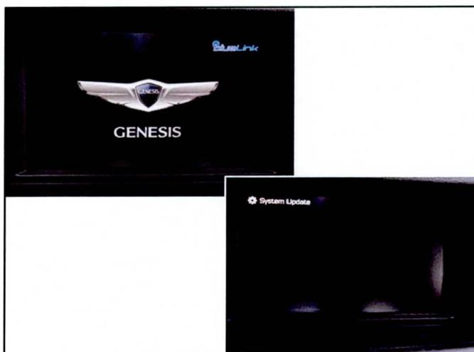
9. If an error code (1312) appears on the screen while downloading the software, press the reset button with a ballpoint pen to continue the downloading process.
