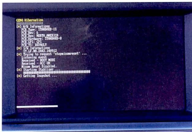
11. After system restart, check the version again following pages 9 to 10. Confirm the version is as shown below.
