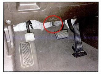
2. Turn the steering wheel left and right full-lock in each direction repeatedly. While doing so, listen and look at the area to identify any noise and/or rubbing condition between the U-joint and the noise isolation pad.
