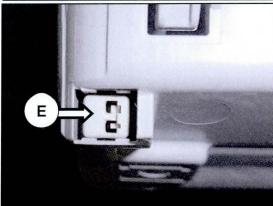
6. Push the back side of the holder latch (E) with a driver (F) to remove the holder latch from the overhead console.
