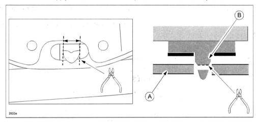
Pull down the reinforcement panel by the masking tape (A) using a suitable tool (B), such as a retaining clip remover, to provide clearance between the reinforcement panel and the remainder of the cut pin. Make sure there is no remaining contact between the pin and the reinforcement panel.
