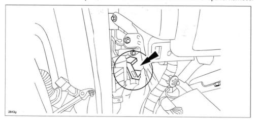
14. Using a small flathead screwdriver, push the tab of the C-08 connector bracket (A) in the direction of the arrows, then remove the C-08 connector bracket from the body.
