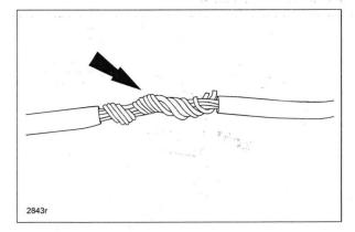
26. Solder the twisted wires together, spreading the solder out across the entire twisted wires.
