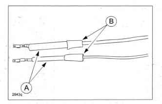
25. Connect the wires from the vehicle side and the wires from the short cord kit by twisting them together.
