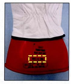
If the glove package has been opened – the gloves MUST be recertified once six months have passed from the date stamped on the glove and every six (6) months, thereafter.
