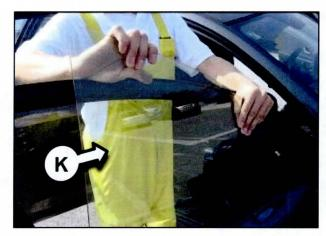
13. Repeat the steps above to install the glass run channel on the opposite side of the vehicle.
