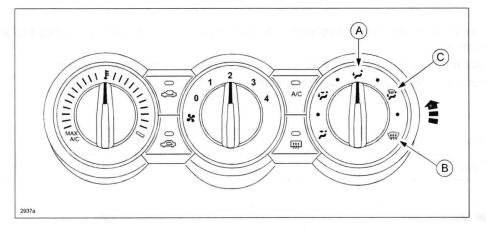
This concern may be due to a production variation. Some of the mode control wires (A) may be too long to transmit movement from the mode selector dial to the link (B). The length of the mode control wire has been shortened to eliminate this concern.
