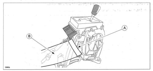
Attach the protector (B) under the protruded area (A) of the selector lever (as shown below).
