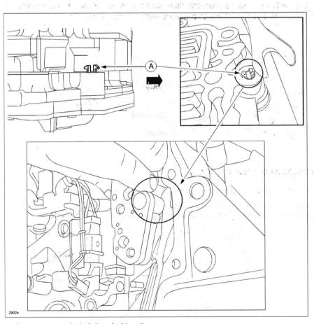
2. Pull out oil pressure switch A by shaking it.
