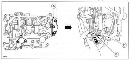
b. Remove the bolts for oil pressure switch A.
