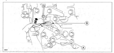
b. Remove oil pressure switch B.
