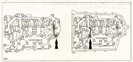
11. Install the oil strainer with new oil strainer O-rings according to the instructions on MS3 online or the Workshop Manual (section 05-17 CONTROL VALVE BODY REMOVAL/INSTALLATION [FW6AEL, FWAX-EL]).
