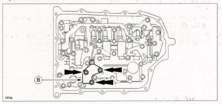
7. Install new oil pressure switches A and B.
