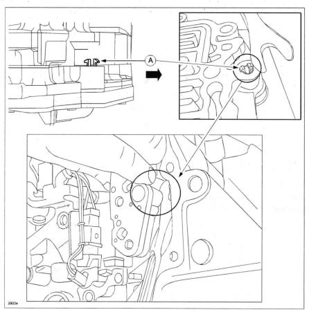
2. Pull out oil pressure switch A by shaking it.
