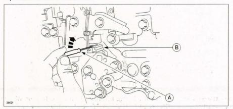
b. Remove oil pressure switch B.
