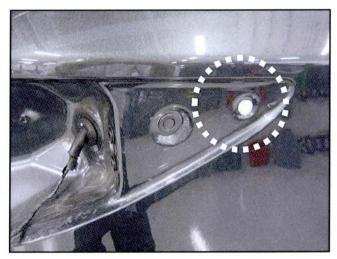
6. Install the new tail lamp. First make the electrical connection and perform a push pull push test to ensure the connection is secure.
