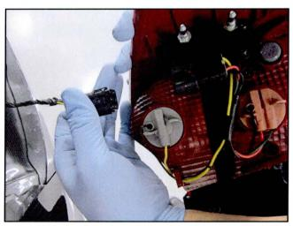
7. Align guide pins and position lamp in to the body. Next push toward the front of the vehicle to secure lamp is in proper position. Finally torque the screws (2) into the pastic mounting bracket then ensure lamp is secure.
