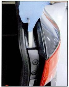
3. With one hand placed behind the bracket and the other hand on the lamp (A), close to the quarter panel. Pull the lamp towards your body until it is free from the vehicle.
