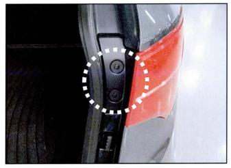
2. Once the screws have been removed place a trim removal tool behind the plastic bracket where the screws were mounted in order to free the bracket enough to position your fingers behind the bracket. This will allow you to pull the tail lamp out of position to be replaced.
