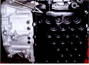
Use a small screwdriver to pry the connector from the oil temperature sensor (except for vehicles with integrated temperature sensor and harness).
