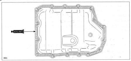
b. Install the oil pan with new bolts before the applied sealant starts to harden.
