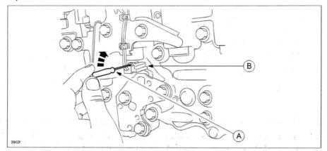
b. Remove oil pressure switch B.
