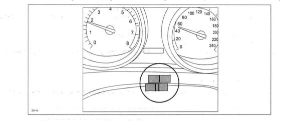
4. Measure the distance between the two lines. The offset can be approximately calculated using 1mm = 1° of offset.
