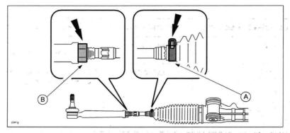
Rotate the tie-rod to adjust the steering wheel center. Refer to the following charts for rotating direction.
