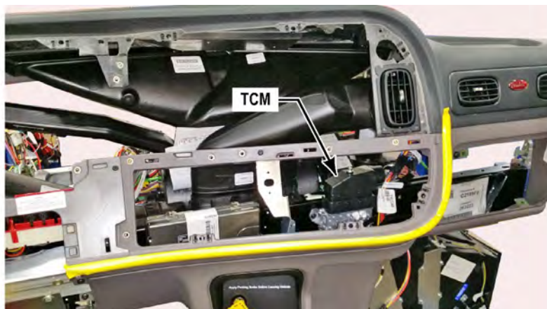
Figure 4. Disassembled Dash Board
