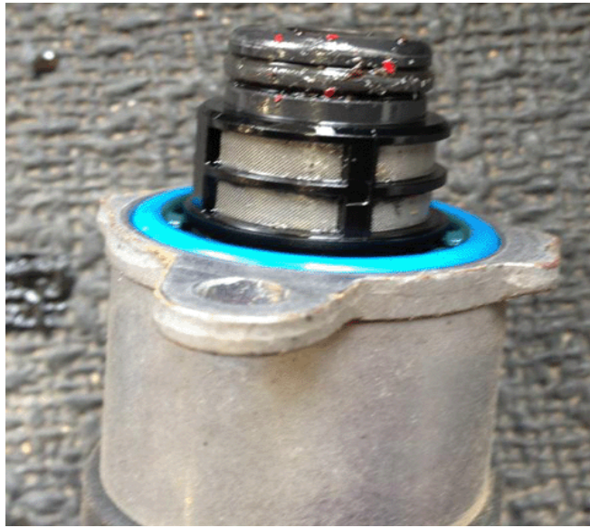
Questionable Fuel Pressure Regulator 1 (View B)
