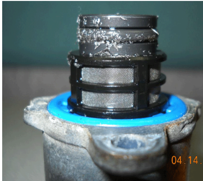
Contaminated Fuel Pressure Regulator 1 (View C)
