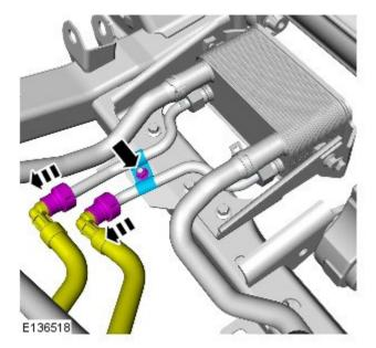
5. NOTE: Use a suitable container to catch any transmission fluid spillage.
