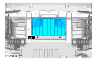
4. NOTE: Use a suitable container to catch any transmission fluid spillage.
