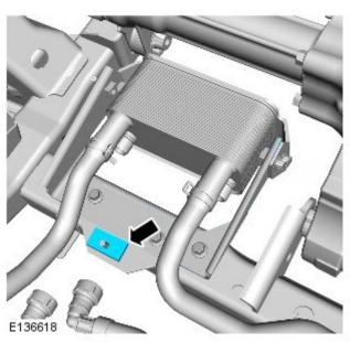
7. Install the two new transmission fluid pipes.
