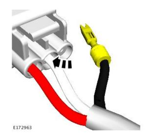
**13.** Install the black wire electrical pin into the right-hand-side socket on the electrical connector.
