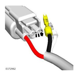
**12.** Install the white wire electrical pin into the center socket on the electrical connector.
