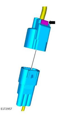
**7.** Using a suitable tool, remove the anti-backout device from the electrical connector.
