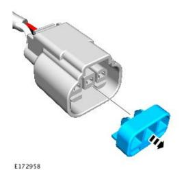
8. Using special tool 418-595, release the electrical connector.
