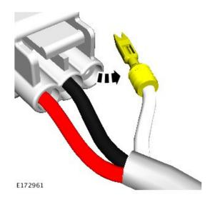
**11.** Remove the black wire electrical pin from the electrical connector.
