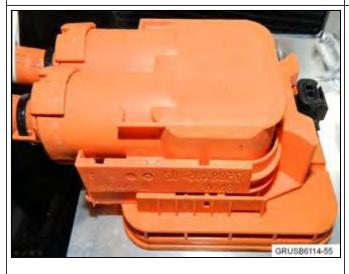
This image shows an HV connector that is properly seated and locked in place correctly.
