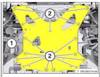
**Note:** Loosen and retorque each screw before starting the next one.
