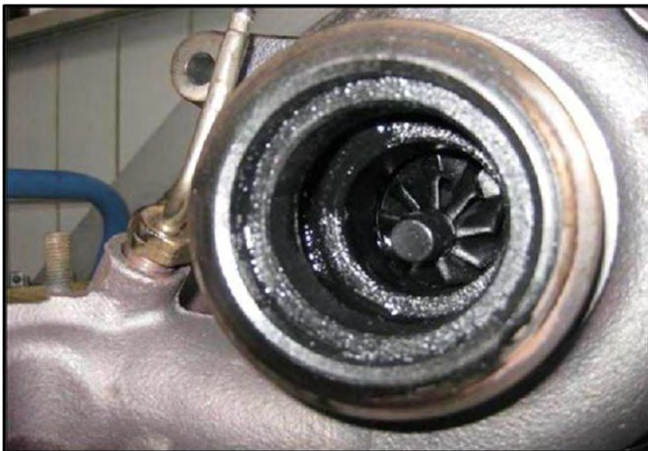
Figure 1 (broken turbocharger shaft, engine oil ingress on exhaust side)
