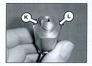
11. Install the Damping Chamber (L) onto the Hydraulic Power Unit (HPU) (M), as shown.
