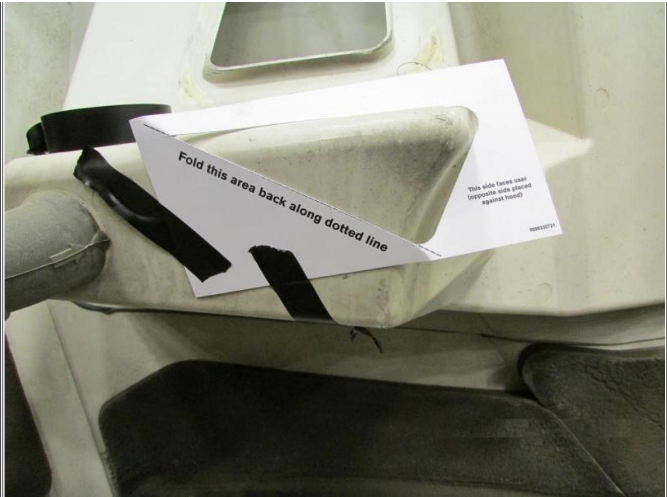
Figure 4: Hood modification template
