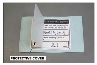
3. Peel off the blue adhesive backing from the decal and then apply the decal to the upper frame tube at the position shown.
