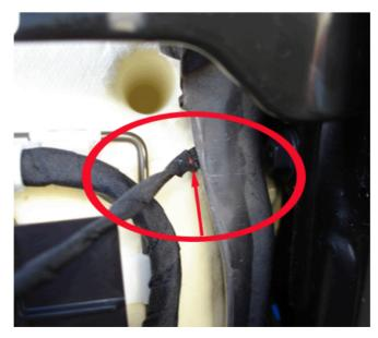
This condition may be due to pressure while sitting in the seat, and the haptic motor wire harness pigtail getting chafed when it comes in contact with the sharp edge of the cushion linkage.
