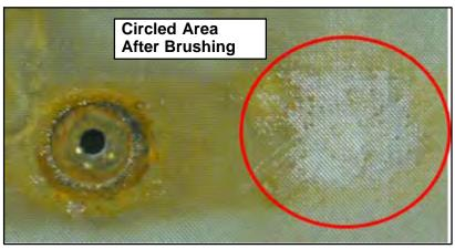
6. Inspect Crossmember A. If rust is present, remove 50% or more of the rust using hand tools such as a wire brush, flat head screwdriver and a scraper.
