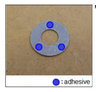
**NOTE:** Apply adhesives to each washer as shown in the left illustration.
