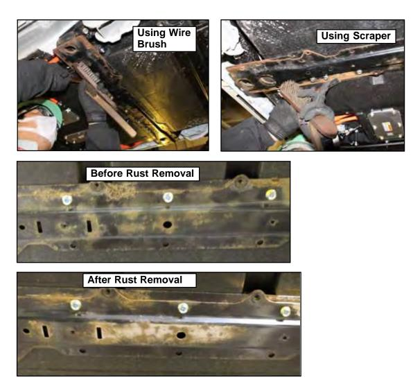
7. Repeat Step 6 for Crossmember B, C, and D and remove rust if required.
