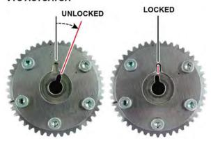
23. Install the new, unlocked VTC actuator onto the camshaft; do not force it on.
