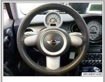
Install the steering wheel so it is straight (turned counterclockwise by seven teeth).
