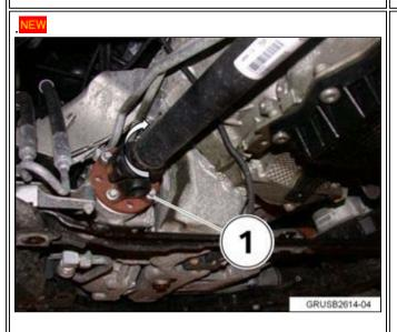
3. Rotate the driveshaft 90° and repeat steps 1 and 2. Rotate the driveshaft another 90° and recheck for play. Rotate a total of four times (the driveshaft has now been rotated 360° total). There should be no excessive play in the U-joints.
