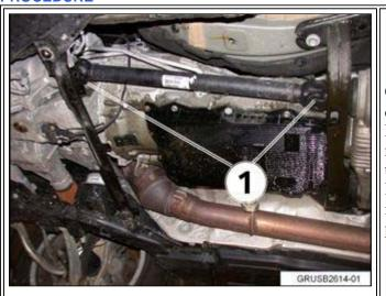
Check the universal joints in the front driveshaft for radial play (1). Note: The E72 will need to have the reinforcement plate removed to check the driveshaft U-joints. Refer to Repair Instruction 31 10 010, "Removing and installing/replacing reinforcement plate."
