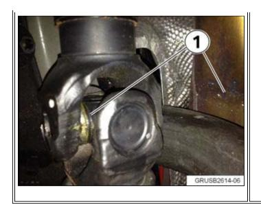
the U-joints and for excessive grease released out of the bearing seals (1).
