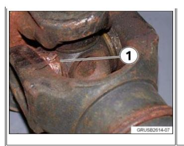
1. New There should be no cracking or damage at the bearing seals (1).
