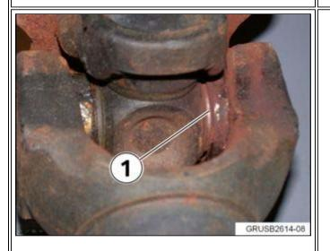
3. New There should be no excessive rust at the bearing seals (1). Note: There will be rust buildup on the driveshaft and mounting flange on some driveshafts. This rust is normal. Only excessive rust on the bearing seals indicates the seal may fail.
