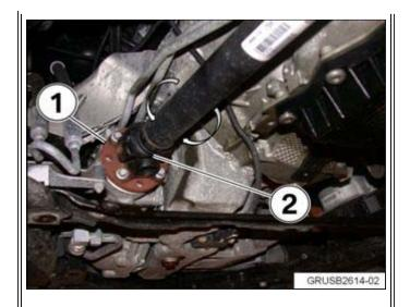
1. Checking the front U-joint:
