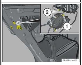
15. Unlock the plug connections (1) and disconnect the cable strap (2).
