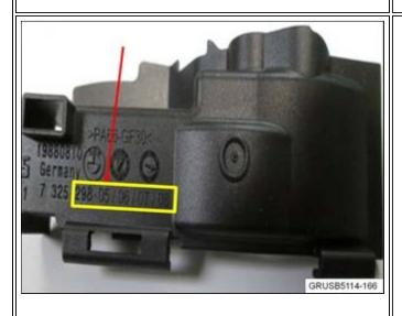
20. Note: The date code on the new Bowden cable cover must be 05 or higher.
