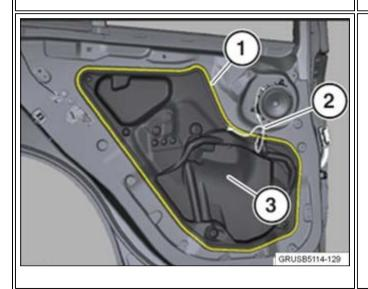
12. Note the position of the sealing bead (1). Pay special attention to the cable (2) when removing the sound insulation (3).
