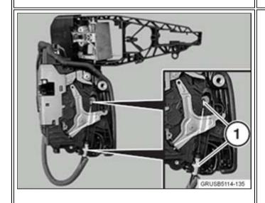
18. Disconnect the Bowden cable (1) and remove the door lock.
