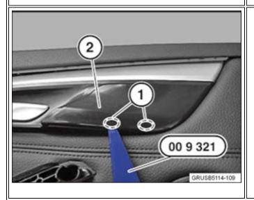
6. Pry the catches in area (1) using special tool 00 9 321. Unclip the trim (2).
