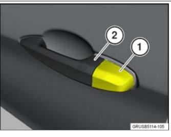
2. Pull the cover off (1) the door handle (2) by opening slightly.
