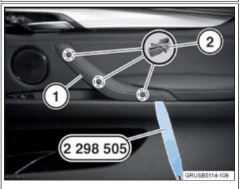
5. Pry the cover (1) from the clips (2) using special tool 2 298 505.
