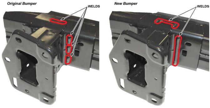
11. Apply a commercially available anti-rust paint like 3M Rust Fighter anti-rust coating (3M P/N 08892) or equivalent to the areas shown, then install the new front bumper beam and torque the bolts to **22 N-m (16 lb-ft)**.
