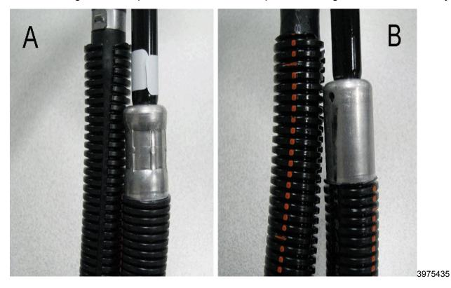
(A) Crimped ferrule with swedge marks. This is a secure connection on the pipe ferrule. (B) Uncrimped ferrule without swedge marks. This is NOT a secure connection on the pipe ferrule.
