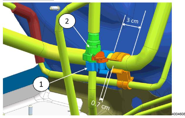
a. Install the swivel clip (1) underneath fuel hose quick connector (2) as pictured above.
