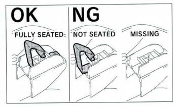
b) Check that the 2 clips are properly installed.
