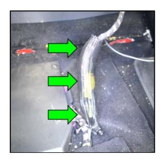
← Reinsert the airbag wiring circuit through the mesh wiring loom <arrows>.
