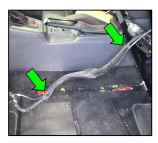
the mesh wiring loom <arrows>.
