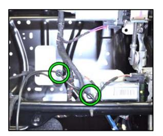
During harness removal, it may be necessary to unfasten the two airbag wiring harness mounting clips <circles>.
