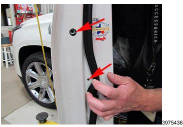
**NOTE**: The left front door may have an anti-tamper bracket around the lock. This is indicated by two screws in the door frame area. Remove these screws along with one internal fastener and reposition the bracket to allow access to the door lock cylinder screw.
