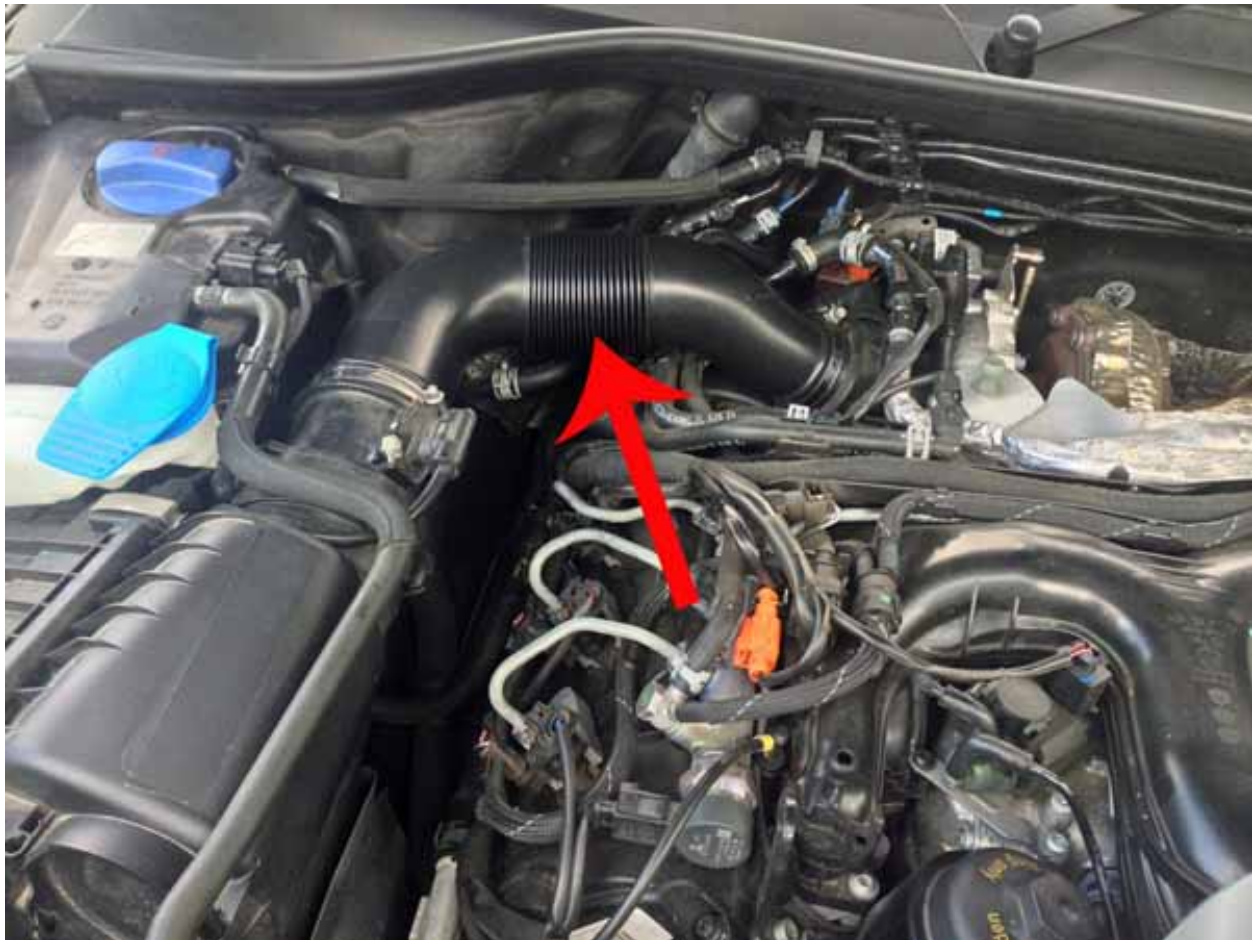
Figure 1. Location of air intake hose
