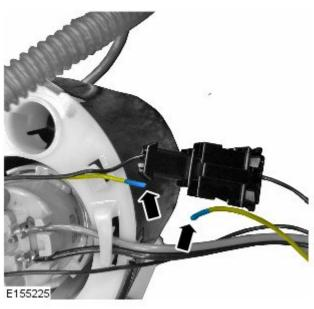
9. CAUTION: After crimping the connection, perform a gentle pull test to make sure that a sufficiently strong connection has been created. If required, remove and replace the splice.
