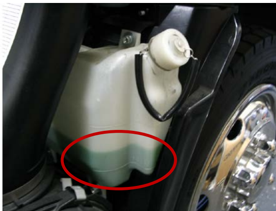
Figure 1 – Without Corrosion Inhibitor
