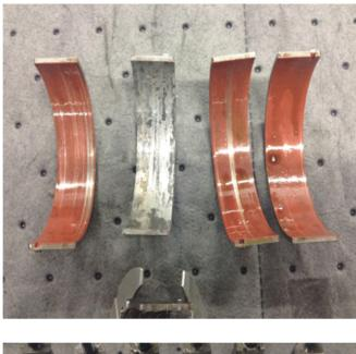
If Due To Bearing Failure when completing diagnosis, and deciding whether to replace the engine or repair it, complete the following before making that determination.
