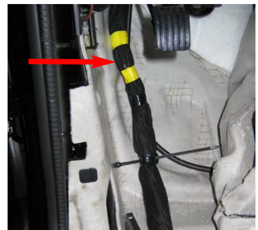
Figure 6 - Tape Marking New Position
