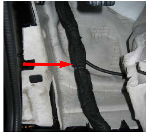
Figure 1 - Main Wiring Harness
