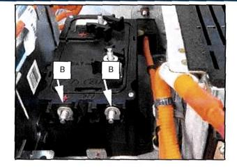
Loosen four nuts (black arrows) and tilt the BMS ECU to the left to provide clearance between the PRA.
