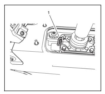
10. Lift to release the shift control neutral lock pin (1).
