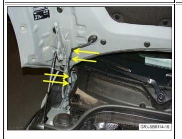
2. Remove the two clips attached to the bonnet and the other two clips attached to the hinge. The picture taken is with the bonnet fully open.
