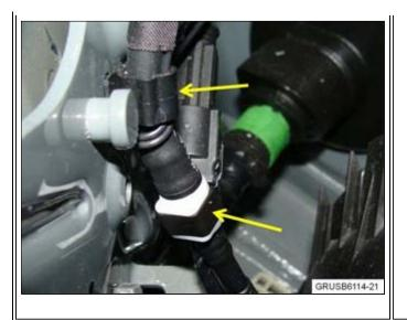
3. At the lower part on the hinge, disconnect the washer hose and the electrical connection. Pull the hose with the clips upwards.
