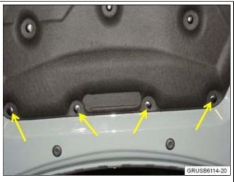
4. Remove the four lower retaining clips from the bonnet insulation.
