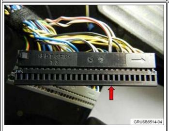
Remove pin 41 (WS/RT) of the grey sub-connector. Install it in the location of pin 87 (BL) of the black sub-connector.
