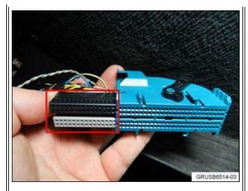
Remove the blue housing of connector A11\*1B to expose the black and grey sub-connectors.
