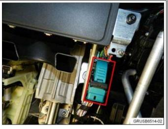
Access the ACSM control module located underneath the steering column, per Repair Instruction REP 65 77 016, "Removing and installing/replacing airbag control unit."
