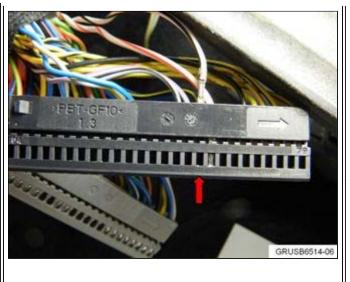
Remove pin 40 (WS/SW) of the grey sub-connector and install it in the location of pin 88 (GR/GE) of the black sub-connector.
