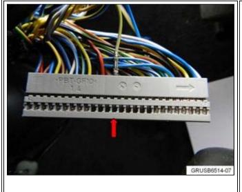
Install pin 88 (GR/GE) of the black sub-connector in the location of pin 40 (WS/SW) of the grey sub-connector.
