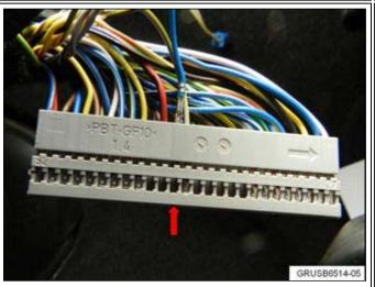
Install pin 87 (BL) of the black sub-connector in the location of pin 41 (WS/RT) of the grey sub-connector.
